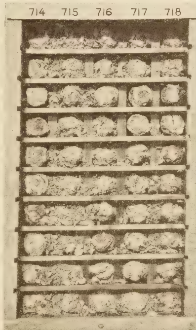
Cylinders made from special cement D and cylinders with Earthcrete admixed, after three years in lake: Series 714.—Special cement D, distilled water 20 days, air 35 days Series 715.—Portland cement, distilled water 20 days, air 35 days Series 716.—Portland cement, 0.27 per cent Earthcrete, distilled water 20 days, air 35 days Series 717.—Portland cement, 1.06 per cent Earthcrete, distilled water 20 days, air 35 days Series 718.—Portland cement, 0.27 per cent Earthcrete, water vapor at 155° F., 48 hrs., air 53 days
